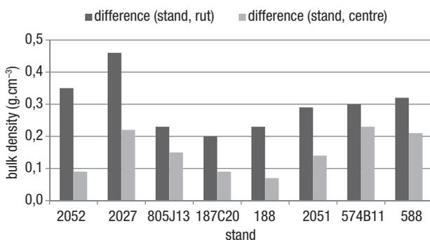
**Figure 4.** Differences in soil densities of dried samples ( $\text{g.cm}^{-3}$ ) caused by different types of chassis in the undisturbed stand, rut and centre of the forwarding line.
