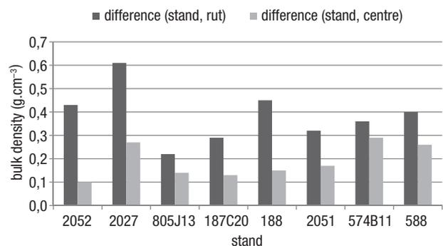
**Figure 1.** Differences in soil densities (g.cm<sup>-3</sup>) in natural conditions (moist) caused by different types of chassis in the undisturbed stand, rut and centre of the forwarding line.
