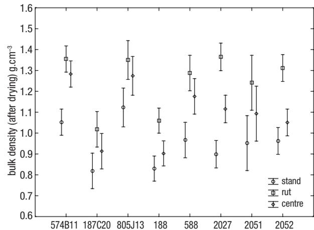
**Figure 5.** Average bulk density of dried samples in individual stands and measurement locations (vertical lines depicting 95% confidence intervals).
