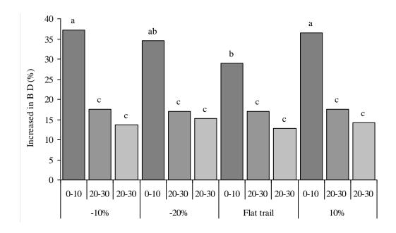
**Supplementary Figure S3.** Average increased in bulk density of four slope gradient in skid trail after different machine passes. Values are mean. Different letters within each terrific treatment shows significant differences by Duncan's test (P < 0.05).
